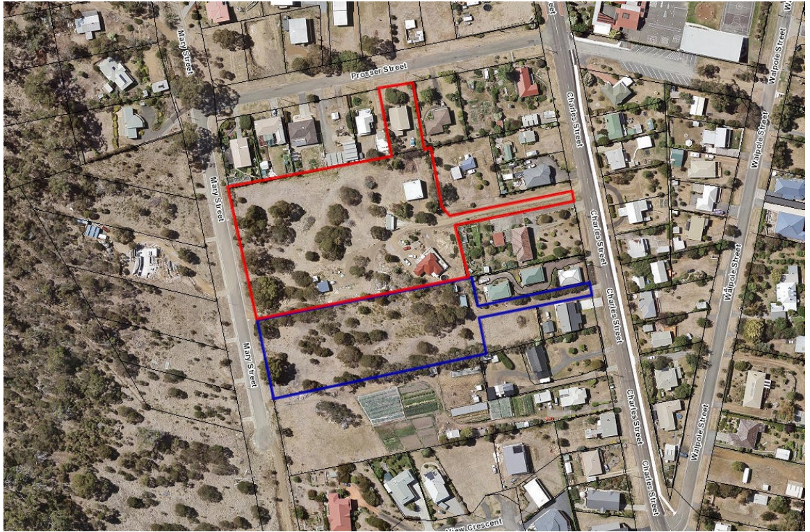
Figure 2 – 52 Charles Street, Orford outlined in blue. Lots subject to the proposed stormwater drainage easements outlined in red (LISTmap)
