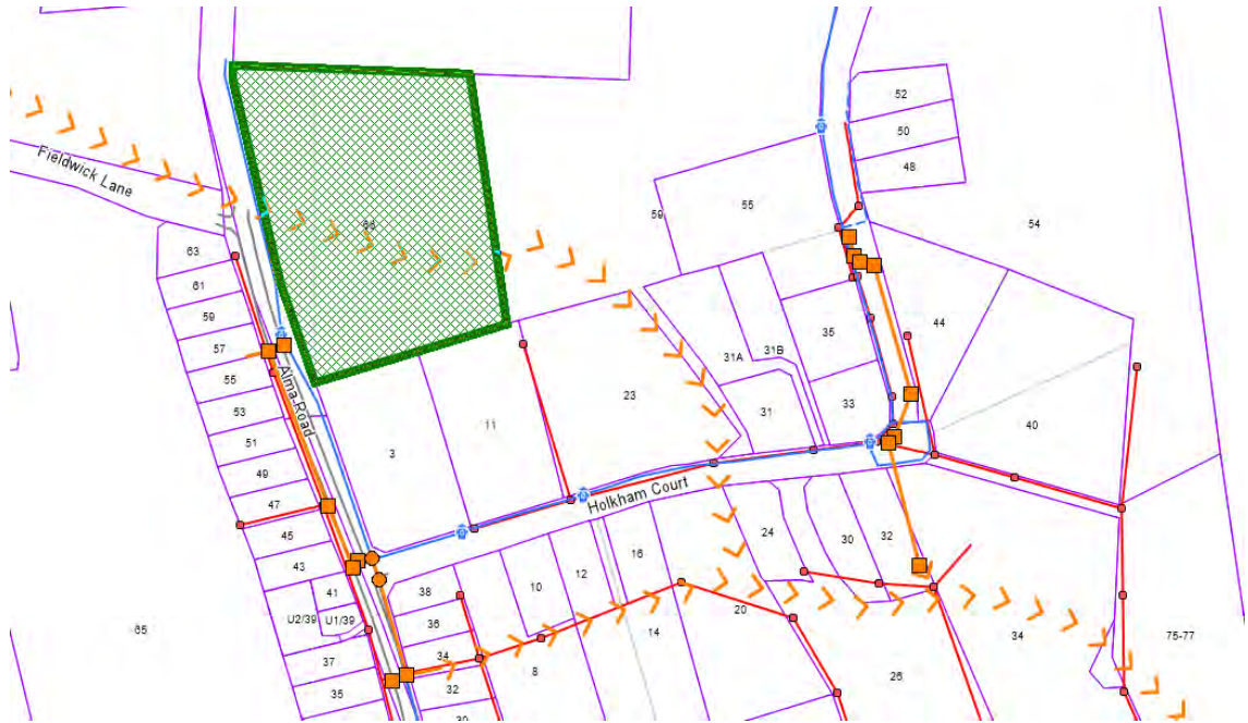
Figure 6: Services. Mains water (blue lines), sewerage (red lines), stormwater (orange lines and orange arrows) (Council's Geographic Information System).
