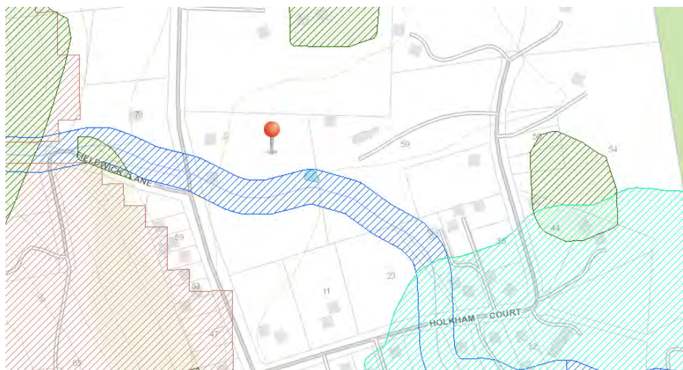
Figure 5: The Waterway and Coastal Protection overlay runs with the waterway from west to east. The pale blue lined area in the south east corner is a Coastal Inundation Hazard Area placed on land below the 10m contour (LISTmap).
