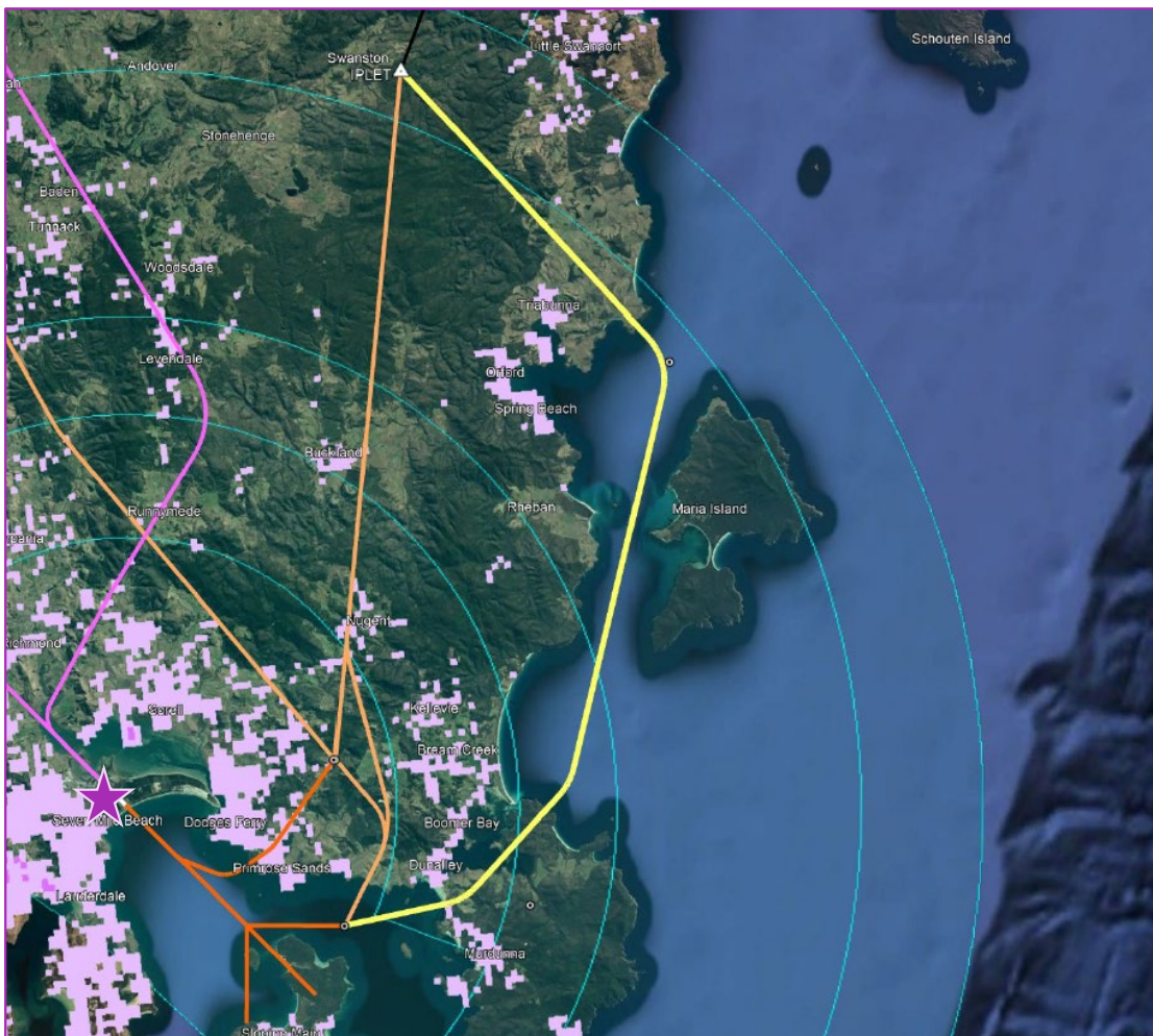
Figure 2: Current arrival path to Runway 30 in orange and suggested over-water arrival path option in yellow . The final approach procedures are shown in dark orange and the departure path that would be used when this arrival is in use is shown in purple . The pink areas indicate population density.
