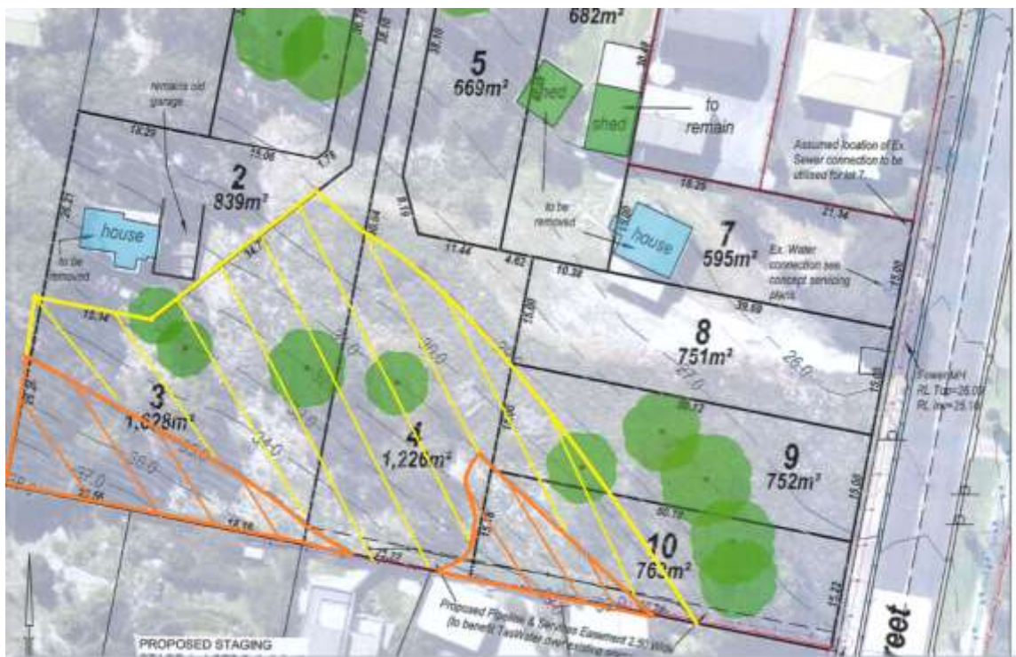
Figure 3 - Approximation of steepness of the site where orange is 20% or higher and yellow is 14% - 20%
