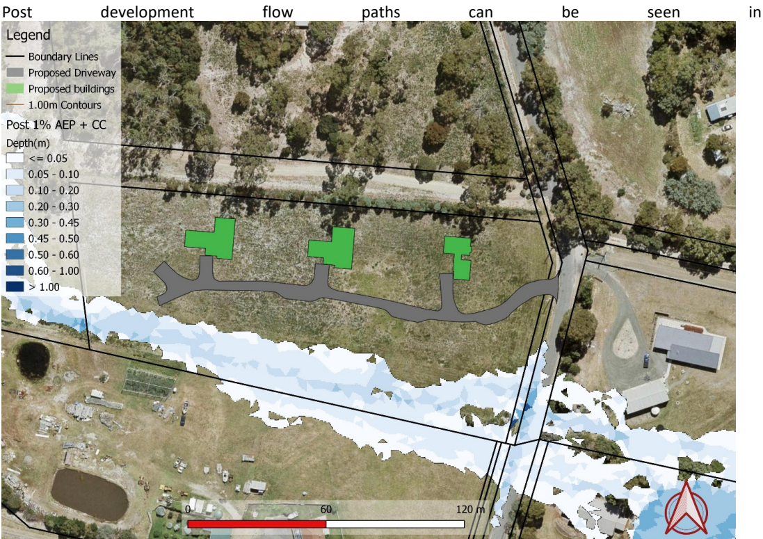
Figure 7. The existing overland flow path shown outside of the proposed development areas and into Harvey's Farm Road.
