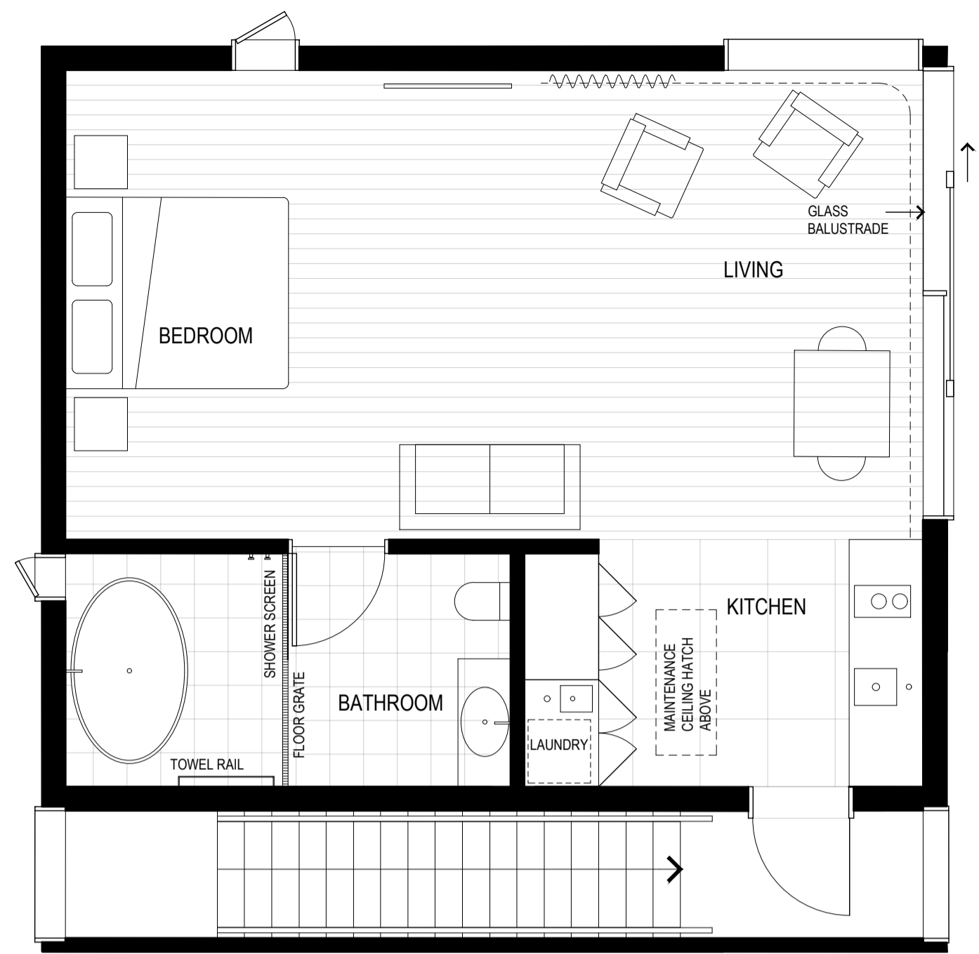
UPPER FLOOR PLAN - TYPE B2 1:100
