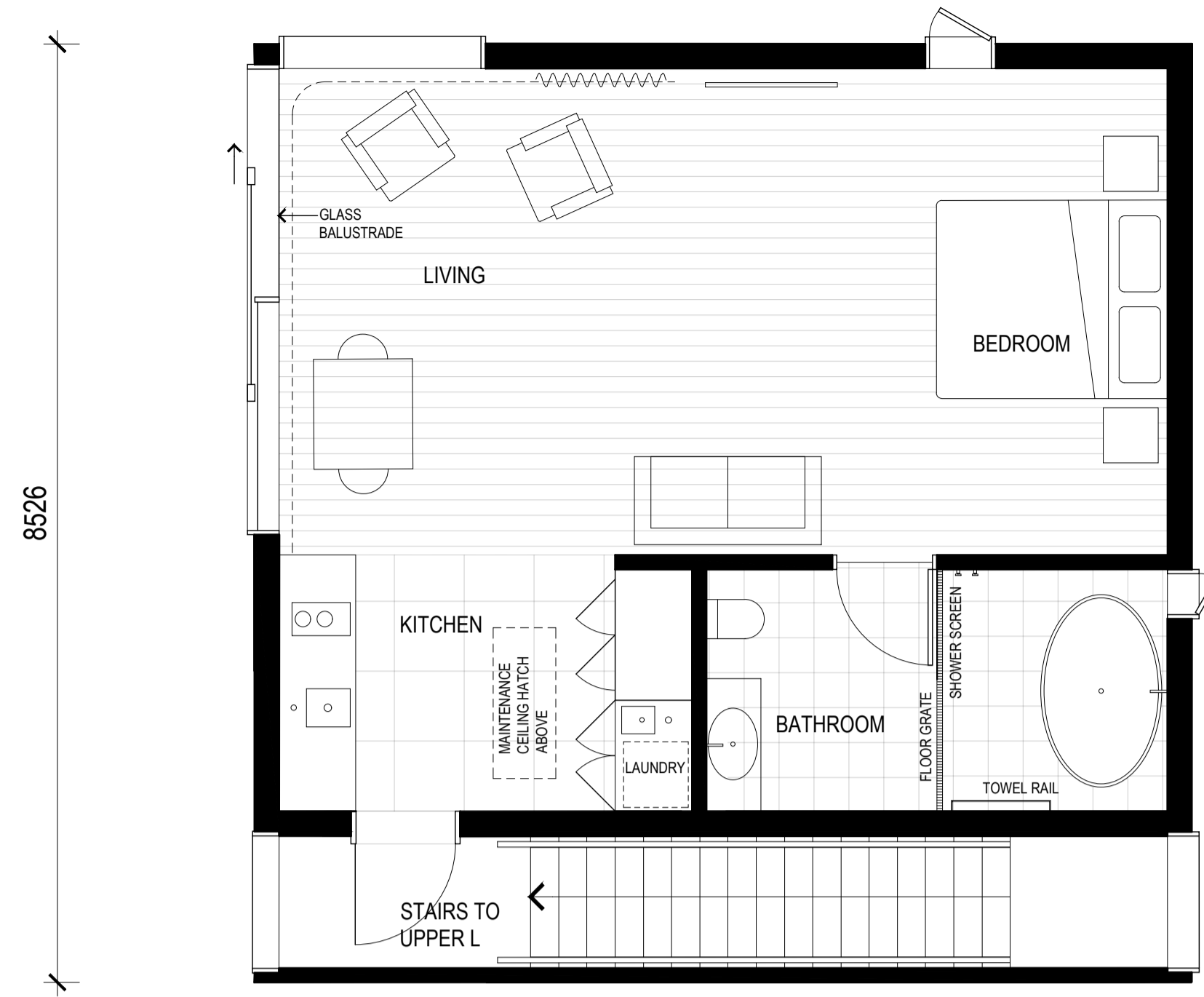
UPPER FLOOR PLAN - TYPE B1 1:100
