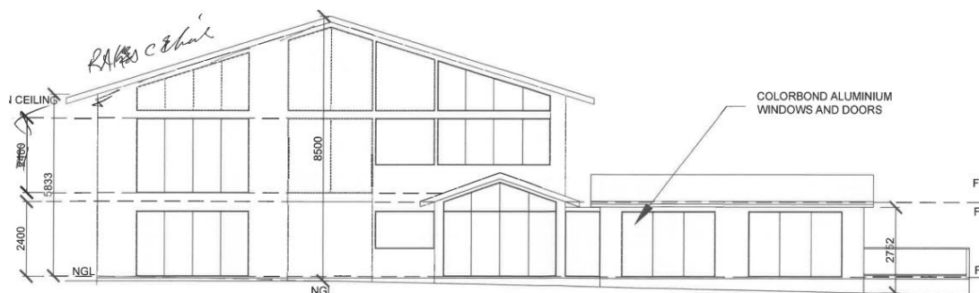
Figure 4: the northern elevation of the approved dwelling. The single storey section is 4m from the foreshore walking track and the double-storey section is 10m from the track.
