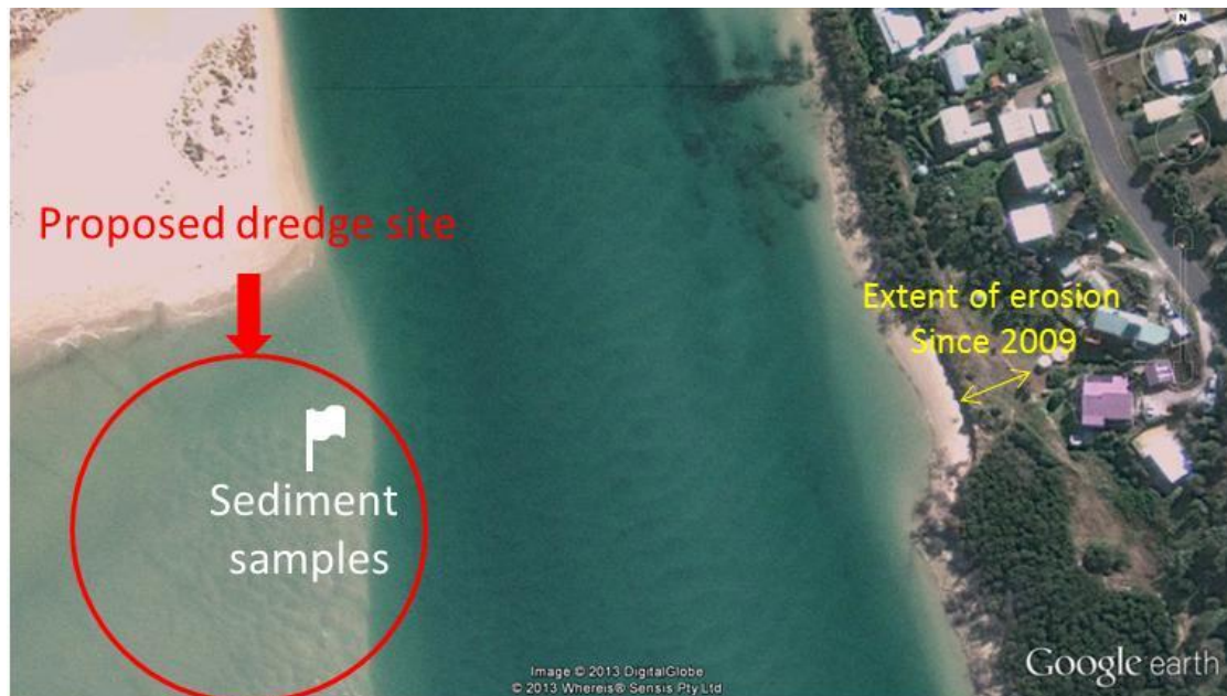
Figure 2 Aerial photograph showing the sandbar of the proposed dredge site; location where sediment samples were taken and; extent of erosion that has occurred since 2009.
