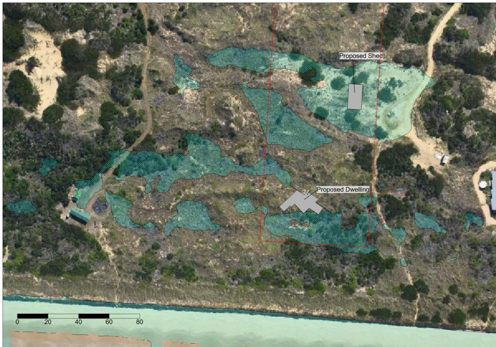
Figure 9 Site Inundation Given a 1% AEP Storm Event for 2065 combined with Wind Setup Conditions
